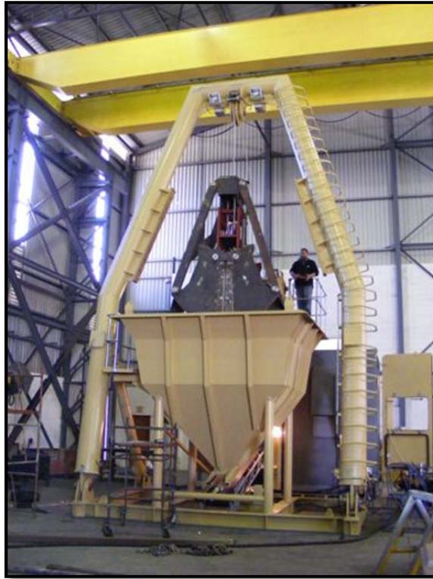
A-frame, 2.0m 3 grab and hopper in the workshop
